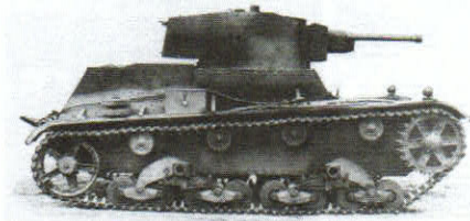
Polish designed 7TP light tank carried a Bofors 37mm anti-tank gun and was the first diesel powered tank to see combat.
